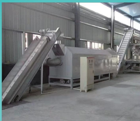
▲ HIGH TEMP HOT AIR FIXATION LINE
